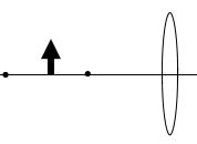
Let's now learn more about magnification (M), image distance (q), and height of the image (h'). The equation for magnification: M = -q/p = h'/h can be split up into: M = -q/p and M = h'/h. h' is negative if inverted (upside down).
