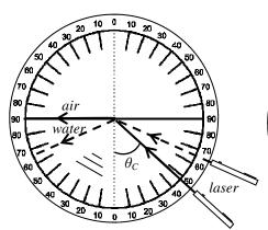
At the **critical angle** ( $\theta_C$ ) the light refracts at 90°, parallel to the surface. Past  $\theta_C$  (example below) he light reflects back into the slower medium. This is known as **total internal reflection**.
