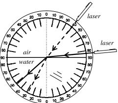
When passing from fast to slow mediums (like air to water) light bends toward the normal, meaning the angle in the slower medium will ALWAYS be smaller. This is why there is no critical angle from fast to slow mediums.
