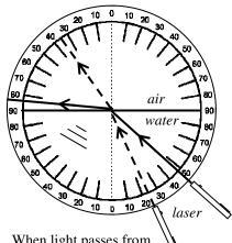
When light passes from a slow medium to a fast medium (like water to air), the light always bends away from the normal and the angle gets bigger. Eventually the refracted light approaches 90°, the surface of the water.
