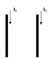
Two current carrying wires interact so that they either attract or repel. Just as a person standing on frictionless ice can't move themself across the ice, a wires can't move itself either.
