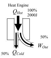
Notice that the  $Q_H$  arrow is equal to the  $Q_C$  and W arrows. So  $Q_H$  is the whole and the others are the parts. W is the useful work done by the engine.  $Q_C$  is the heat that is not used, so is "wasted" and is the inefficiency of the engine. This engine is 50% efficient.
