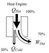
This engine is more efficient because less heat is lost at  $Q_C$  and the useful work is a greater percentage of the absorbed heat  $(Q_H)$ . This engine is 70% efficient. Only 30% is lost to the environment.
