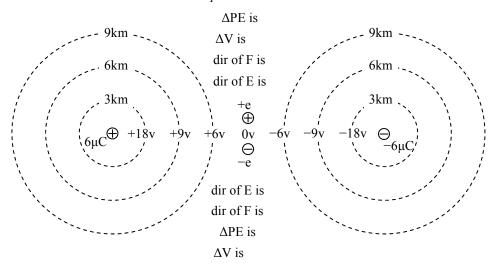
I have now put all of the potentials (voltages) on the diagram for you, to simplify the following discussion. Notice that I have placed a +e and a -e at the 0V point. The +e stands for a positive elemental charge: a proton. The -e stands for a negative elemental charge: an electron.
