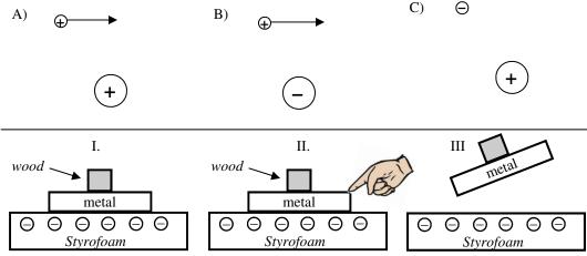
4. On the diagram above, the Styrofoam has been made negative by rubbing it with fur. A. In the picture I, draw where the negatives are on the metal.
