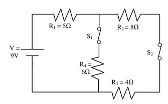
7. Now, switch 1 is opened. Calculate the new current and voltage used by the  $8\Omega$  resistor.
