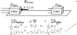
\* A 6 kg object is moving 4 m/s to the right. A 3N force slows the object down to 2 m/s.
