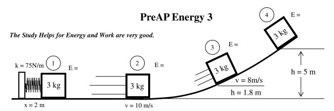
1. A 3 kg object is against a compressed spring. When released the object moves up a ramp until it stops. Assume there is no friction on the surface and use  $g = 10 \text{ m/s}^2$ .
