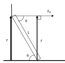
Torque = perpendicular force times distance:  $\tau = F_{\perp}d$ .
