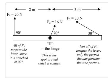
To find the net torque add up all of the torques:  $\Sigma \tau = \tau_1 + \tau_2 + \tau_3 \dots$  Where  $\tau = Fdsin\theta$ ; F is the force; d is the distance from the rotation point (H);  $\theta$  is the angle from the lever and the force.
