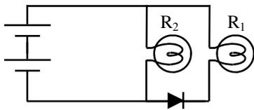
10. In the circuit at the left, R<sub>1</sub> isn't working. Without doing anything to the light bulbs, what is one change that would make R<sub>1</sub> turn on?
