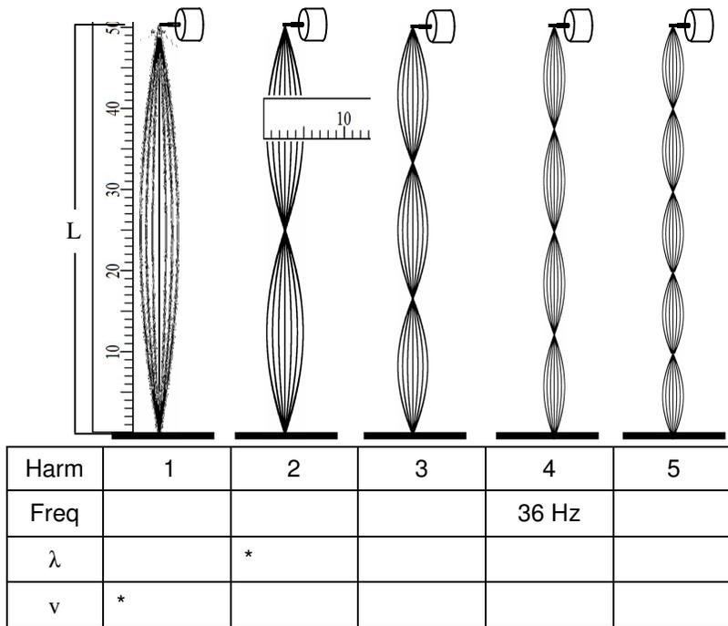
1. A mechanical vibrator is attached to an elastic string. At particular frequencies it forms the given shapes.
