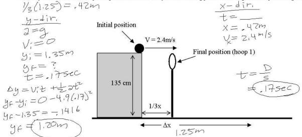
C. Calculate the angle of hoop 1 by finding Vx and Vy at the hoop.
