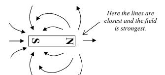
3. The magnetic field of a magnet or solenoid is strongest closest to either of the poles OR, for a solenoid, inside the solenoid. Just like for electric fields, the field is strongest where the lines are closest.
