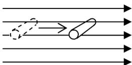
In the example at the left the magnetic field lines are pointing to the right and the wire is moving to the right. The wire is NOT breaking the magnetic field lines: it is passing between them. So no current is induced in this wire. OR, by the RHR, the wire ( $q$ , thumb) and  $B$  (fingers) are in the same direction, so no force (palm)
