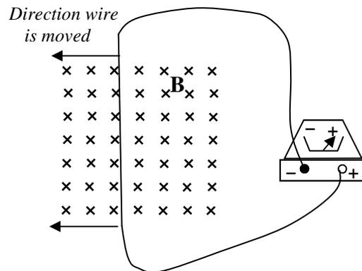
1. Let's learn what part of the right-hand rule is a moving wire. The diagram at the right shows a wire being moved to the left by an external force (like a person).
