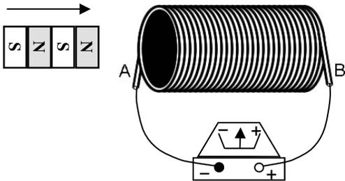
3. The north pole of a stack of magnets is moved into a solenoid.
