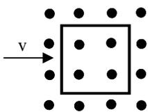
So, since the loop is entirely inside the field, there is no change of  $B$  in the loop, so there is no  $I_{\text{induced}}$  and no  $B_{\text{induced}}$  in the loop.
