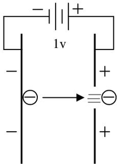
An electron repelled by a negative plate and attracted by a positive plate has potential energy. Since volts = J/C, then PE = qV. This potential energy becomes kinetic energy, so that  $qV = \frac{1}{2}mv^2$ .
