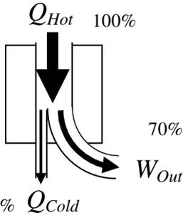
Again, on the diagram, notice that  $Q_H$  is 100%.  $W_{out}$  is the efficiency. This diagram shows that the efficiency is 70% (which =  $W_{out}$ ). The inefficiency is  $Q_C$  (or 30% for the engine). This allows you to do very simple proportions.
