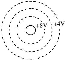
3. The dashed lines on the diagram at the left show the equipotential lines (which you should now recognize) around an unknown charge.
