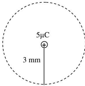
1. Calculate the four electrostatic quantities (E, F, PE, and V) 3 mm from a  $5\mu\text{C}$  charge, as shown in the diagram. Be sure to give direction, if necessary. Some may be zero. Notice, keeping  $r$  constant produces a sphere that is 3 mm away from the  $5\mu\text{C}$  charge. This means E, F, PE, and V will have particular values everywhere on that sphere.
