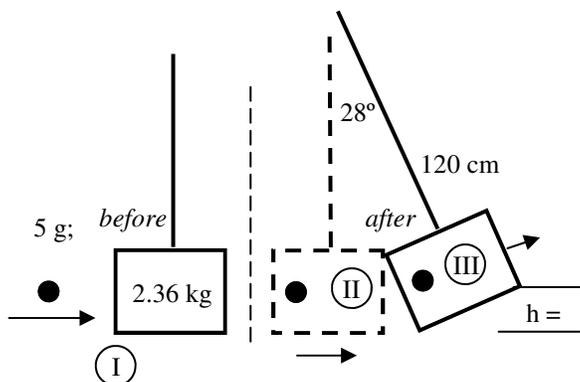
3. A ballistic pendulum is used by forensic scientists to determine the speed of bullets. Let me walk you thru how.
