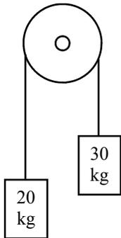
3. Two masses are suspended from a frictionless, massless pulley. Following the "Connected Object and Ramps" notes exactly, calculate the \* acceleration and tension in the rope.
