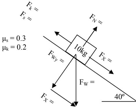
1. A 10 kg object is placed on a ramp that is tilted at  $40^\circ$ .
