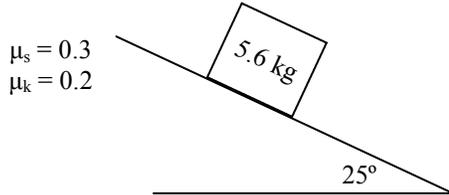
2. Now a 5.6 kg object is placed on a ramp that is tilted at  $25^\circ$ .
