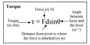
Torque is a twist around an axle. Only the portion of the force perpendicular to the axle gives torque. In gears the force is always at an angle of 90°, so  $sin\theta = 1$  and can be ignored.
